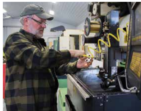
AUTOMATED MACHINING: J&S Precision Machining owner Steve Sweeley uses compressed air to clean a key hole die created using a manufacturing process known as wire electrical discharge machining. The computer-automated process uses electrical discharges through a thin brass wire to create shapes in hardened tool steel.
